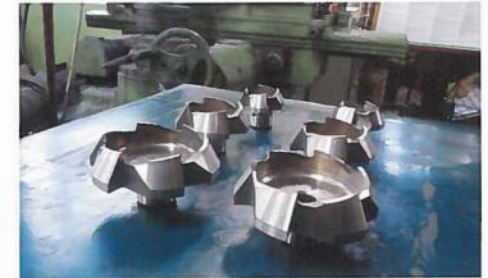
New purpose-made cutters from Somta Tools that were used in the extraction of the infected tusk
